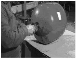
Unscrew the valve cap and gradually release the internal pressure
