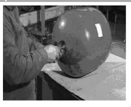
Insert the new membrane rolled up inside the tank, holding the neck of the membrane against the flange
