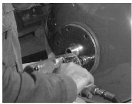
Once the pressure is released, unscrew the nuts of the blocking counterflange and remove it;
