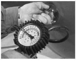
Restore the precharge of the tank according to the value specified on the label of the tank
